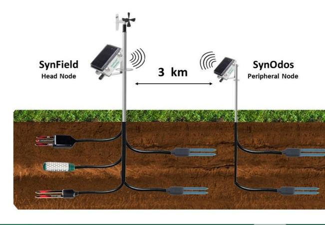
The interconnection between SynField and SynOdos device is based on the LoRa wireless technology. The distance between **SynField** head node and **SynOdos peripheral** node can reach **up to 3 km.**
